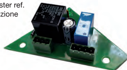
00800208 FEEDING EL. BOARD FOR DAIRYMASTER REF. DM917A
